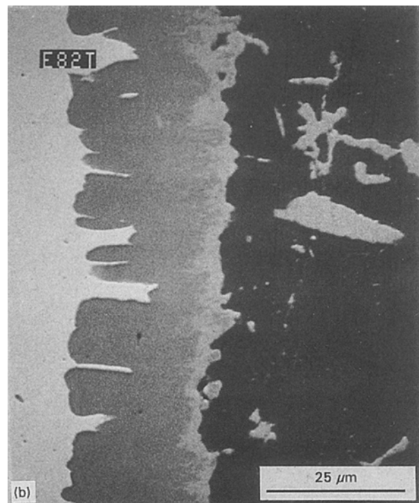
Figure 6 Intermetallic layers after dipping XC18 insert in AU5GT alloy, 750 °C, 18 s, 50 MPa. (a) not heat treated; (b) heat treated.
